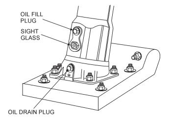
Figure 15. Oil Drain Plug
